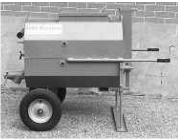
The 55-gallon Patch Kettle, the 55-gallon Insulated Tank and the 55-gallon Insulated Patch Pot may be used with either the utility carrier or the stationwagon carrier. Channel irons securely attach the tank on either carrier.
