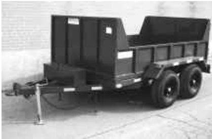
TR100 HD (regular size sides) Planks slide in side holders to increase wall height
